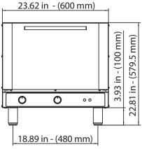
\* Oven must be installed a minimum of 19.7" (500 mm) from any significant source of heat and/or grease (for example: fryers, burners, kettles, open flames, etc.)
