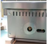
3. Replace the orifice fittings into the valve. **Note:** Unit Number on side of orifice fittings.
