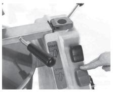
PRESS RED STOP BUTTON. A built-in brake will quickly stop the attachment shaft when power has been turned off.
