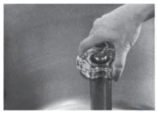
5. LOCK ATTACHMENT. Use the twist lock knob furnished. Simply line up the notch on the knob with the notch on top of the attachment shaft. Place knob over shaft and push down until flush with top of shaft. Twist in either direction until tight.
