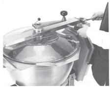
2. UNLATCH COVER. Holding cover handle in left hand, pull the cover latch toward you.
