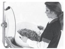
REMOVE STRAINER BASKET. Grip handles and raise strainer basket. Drain and transfer product. The bowl water can be re-used for another batch.
