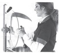
6. INSERT MIXING BAFFLE (WHEN REQUIRED). With the cover still upright, hold the baffle in right hand with scraper at bottom. Insert baffle shaft through hole cover. Press firmly against cover.
