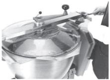
UNLATCH AND OPEN COVER. Be sure to wait until shaft has stopped turning.
