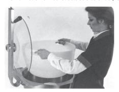
1. **INSERT STRAINER BASKET.** Do *not* use the mixing baffle when using the strainer basket.
