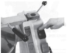
2. PRESS START SWITCH AND HOLD. Machine will run until switch is released.
