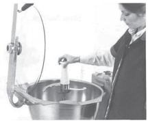
4. INSERT ATTACHMENT. Slide attachment onto center shaft. Rotate until it drops down over square part of center shaft. Make sure attachment drops completely into place.
