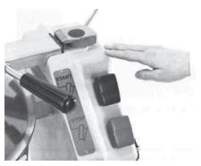
RELEASE START SWITCH. Machine will automatically brake to a stop. Continue pressing the start switch for as many on-off bursts as necessary.
