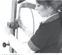
8. LOCK BAFFLE. Rotate lock knob downward until it stops.
