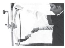
SCRAPE COVER AND MIXING BAFFLE. The cover scraper will remove most product from the cover. To remove remaining product use rubber scraper.
