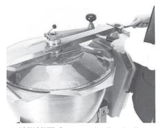
LOCK COVER. Grasp cover handle and pull cover down into closed position. Press cover handle down before rotating cover latch away from you.
