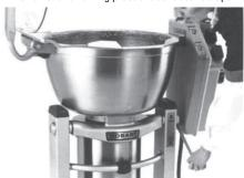
5. UNLOCK BOWL. Lower the bowl tilt lever to the "Tilt" position.
