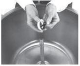
12. CLEAN BOWL SEAL AND RETAIN-ER RING. Bowl seal and retainer ring easily snap on and off without tools. Wash if necessary, and dry. Replace and close cover.
