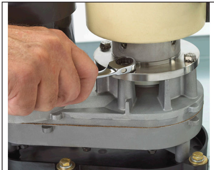
Remove Evaporator Bolts
