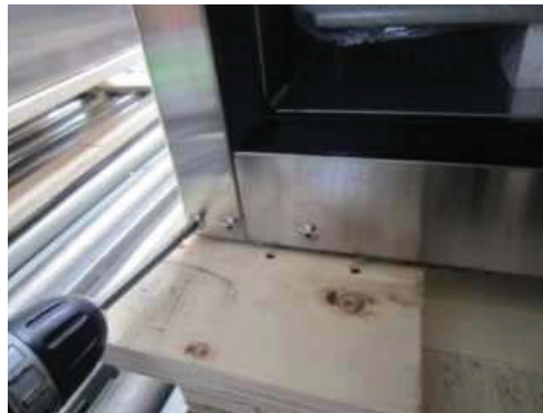
C-2. Disassemble bottom hinge (left).
