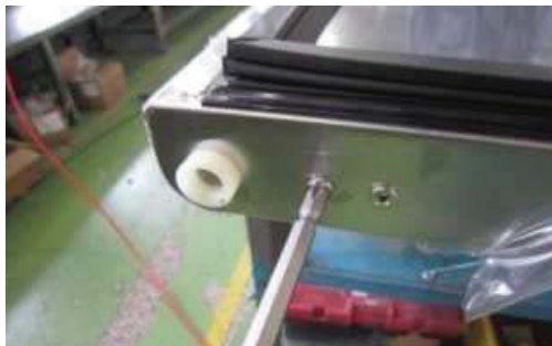
F. Disassemble stopper plate, then tight screws.
