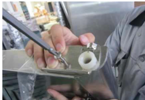
G. Assemble stopper plate in original positions.
