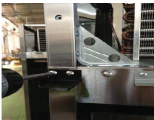
C-1. Disassemble the top hinge (left).
