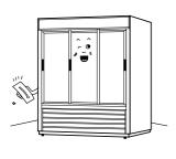
■ Set the front of the refrigerator a little bit higher than back-side by using adjustable feet to drain the water away with easily.
