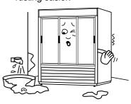
Ambient temperature should be below 85°F. Warmer temperature will cause problems with cooling efficiency.
