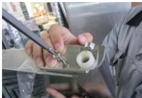
G. Assemble stopper plate in original positions.
