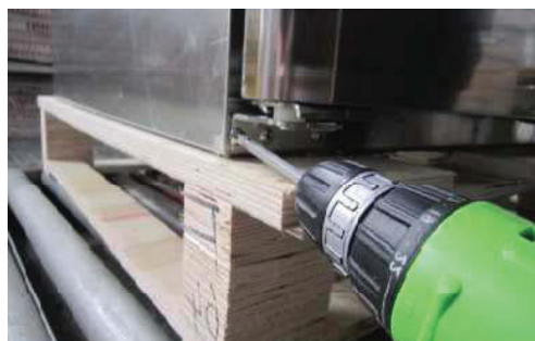
H. Assemble the door, then rotate it about 180 degrees. Assemble top hinge (right) with stopper plate in bottom hinge (left) position (First, assemble top hinge (left); second, assemble bottom hinge (left) while doors are closed, insert hinge into door bushing (left) with lifting, rotate doors counter-clockwise, screw hinge in original positions).
