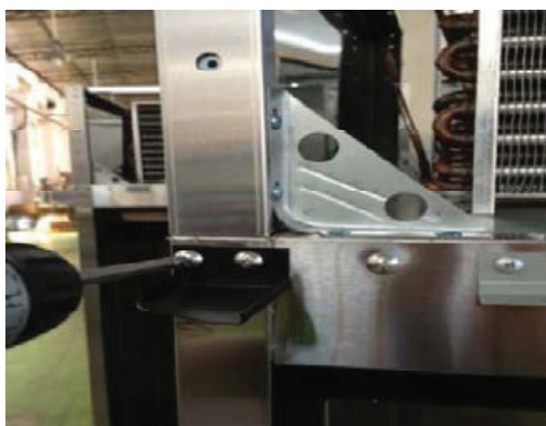
C-1. Disassemble the top hinge (left).
