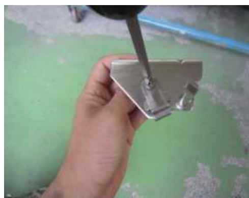
C-2. Disassemble bottom hinge (left).
