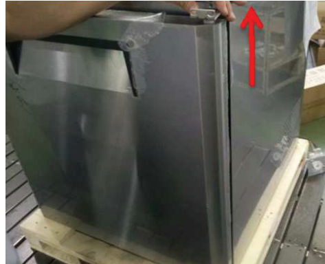
2) Remove the top hinge from the unit.
