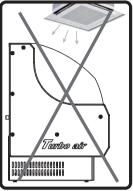
Units should not be placed near HVAC vents.
