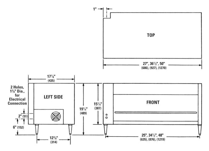
(Measurements in parenthesis in millimeters) \*Leave 3" clearance on the left side for air movement.
