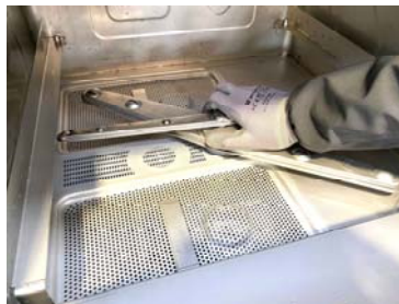
Unscrew the lower rinse arm
