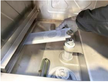
Remove the central support
