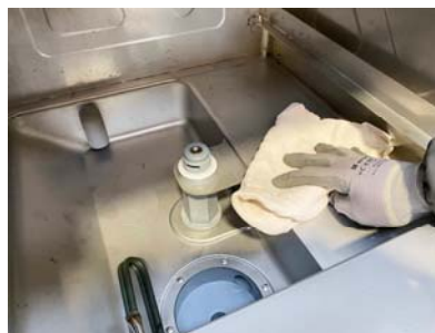
Remove from the tank by means of a brush or cloth if any, residual dirt.
