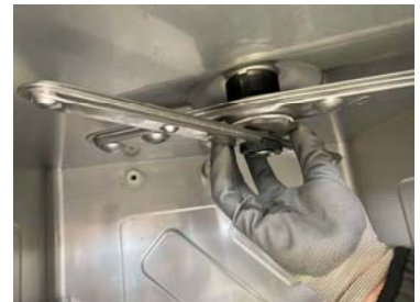
Remove the rinse arm on the top
