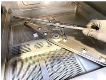
Remove the lower rinse arm
