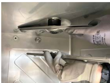
Remove the washing upper arm
