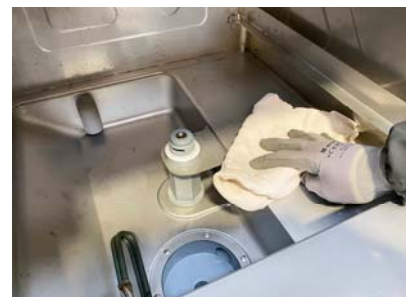
Remove from the tank by means of a brush or cloth if any, residual dirt.
