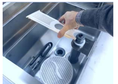
Remove the central support
