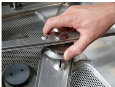
Unscrew the reel rinse lower
