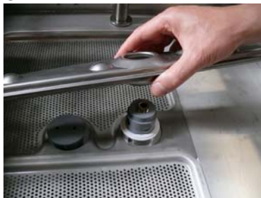
Remove the washing lower reel
