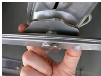
Unscrew the reel rinse top.
