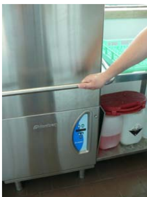
Completely close the hood the the dishwasher. If there is an extended downtime, it is advisable to leave the hood open.
