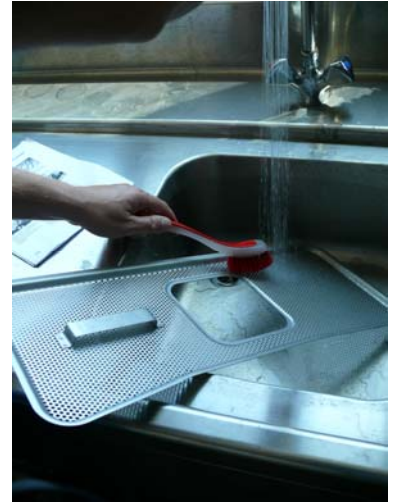
Clean the filter tank top
