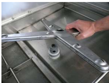
Remove the washing lower reel
