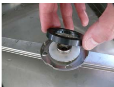
Control the wear washer cod.0201558 of the upper rinse arm is in his place.
