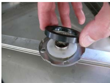
Control the wear washer cod.0201558 is in his place.
