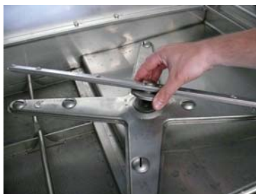
Screw the lower rinse arm
