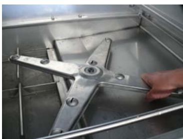
Replace the lower washing arm
