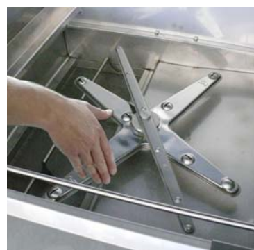
Check that the wash and rinse arms are free to rotate (upper and lower)
