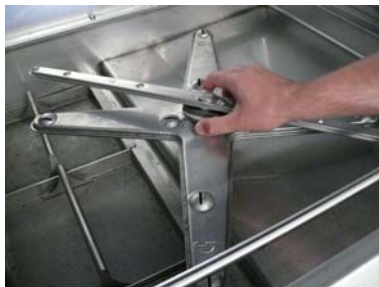
Unscrew the lower rinse arm
